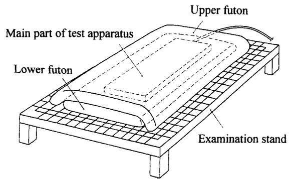
Fig.2 Futon heat retention performance test apparatus
