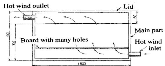
Fig.9 Futon humidification and drying apparatus High-speed drier
