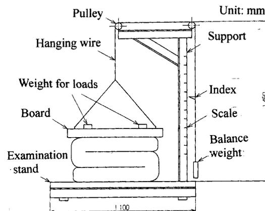
Fig.4 Resilience test apparatus for futon finished products
