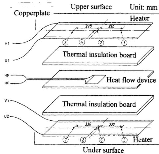
Fig.3 Main part of futon heat retention performance test apparatus (Patent)
