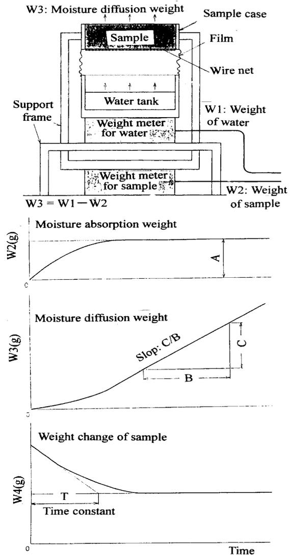
Fig.8 Moisture transfer characteristics (Moisture transfer characteristics test apparatus from a top, futon absorbency, moisture diffusion and moisture permeability) (Patent)
