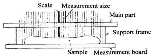
Fig.7 Form measurement instrument for futon finished products
