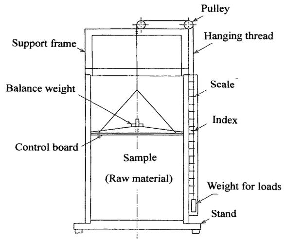
Fig.5 Resilience test apparatus for down (raw materials)
